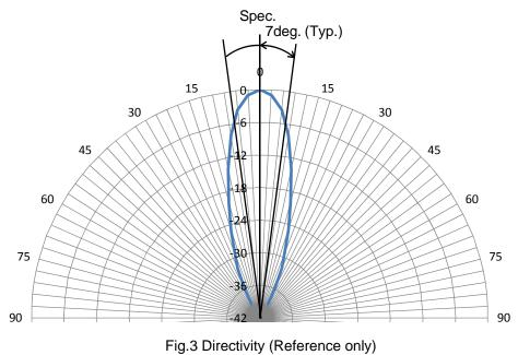
(note) Directivity is defined the half-angle of the half sensitivity (-6dB) against peak sensitivity.
